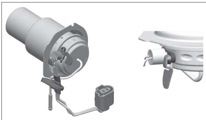
Fig. 30 Glow plug correctly mounted
