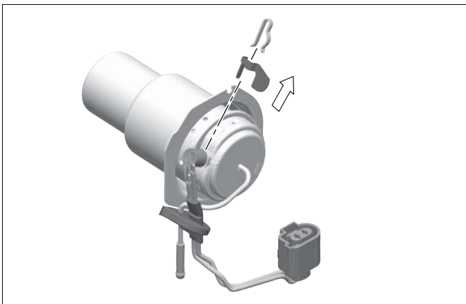
Fig. 25 Disassemble cooling flag
