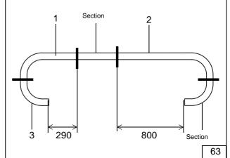
Cut the second supplied water hose into three sections, as shown in figure 64:
