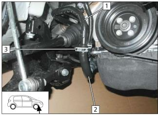
▶ Remove heat exchanger outlet / engine inlet hose 2 at position 3 from heat exchanger outlet hose 1. Original vehicle spring clip 3 will be reused.
