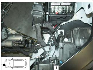
▶ Route heater wiring harness **1** along the marking to the radiator and fasten using a cable tie.
