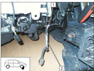
▶ Mount 180mm long heat protection tube 2 as shown, starting at the cable tie at position 1.
