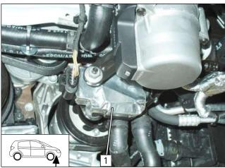
▶ Apply self-adhesive heat shield to original vehicle 3-way valve 1 as shown.
