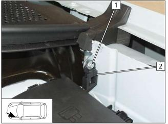
1 M5x16 bolt, large diameter washer, retaining plate of SH2, angle bracket, large diameter washer, nut
