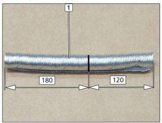
► Slit the heat protection tube lengthwise open and cut it to length as shown in Fig..
