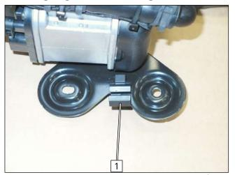
1 Original vehicle wiring harness bracket
