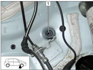
▶ Open original vehicle pass through **1** in the centre as shown.
