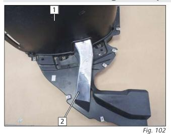
► Glue heat protection film 2 on wheel-well inner panel 1 as shown.
