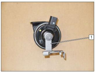
▶ Remove and discard horn bracket 1. The nut will be reused.
