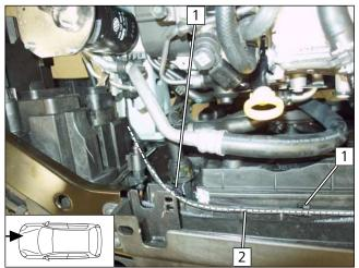
▶ Route heater wiring harness 2 along the marking to the heater installation location and fasten using edge clip cable ties 1.
