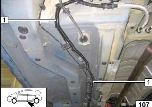
Route fuel line and wiring harness of metering pump in corrugated tube **1** to the installation location of the metering pump.
