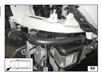
Align hoses. Ensure sufficient distance from neighbouring components.
