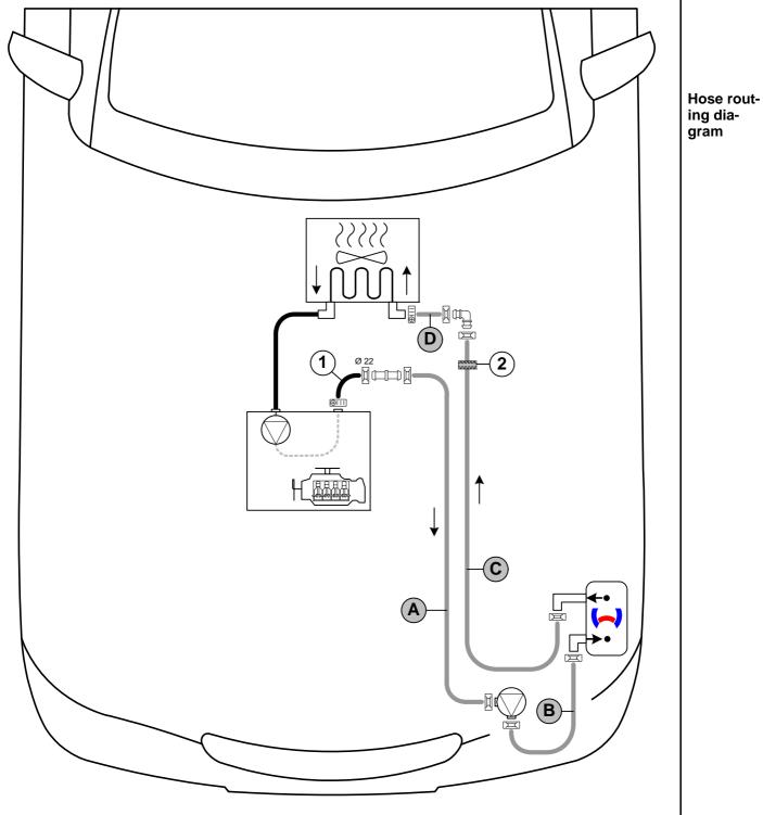
All spring clips  $\square = 25$  mm dia. All hose clamps  $\bigcirc 111 = 20-27$  mm dia. **1=** Original vehicle hose **2** = Black (sw) rubber isolator  $\blacksquare$ . Connecting pipe  $\blacksquare = 18x18$ mm dia. Connecting pipe  $\square = 15x18$ mm dia.
