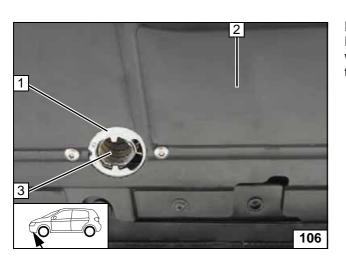
Install engine cover **2**. Install exhaust end section **3** according to work step 6 - 8 of the installation instructions.
