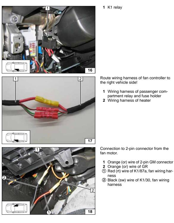
Connecting same colour wires of wiring harness-
