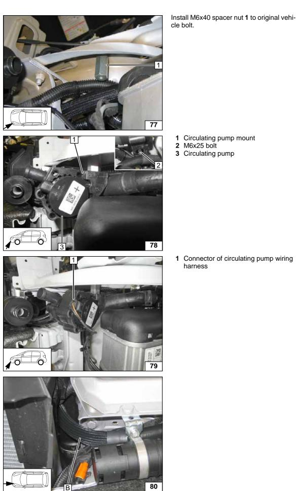
Installing spacer nut Installing circulating pump 1 Connector of circulating pump wiring Installing wiring harness
