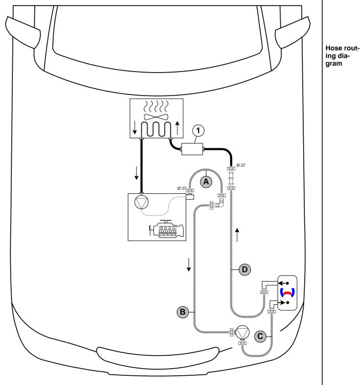
All spring clips without a specific designation  $\square = 25$ mm dia. Connecting pipe  $\square = 18x18$ mm dia. Connecting pipe  $\square = 18x20$  mm dia. **1** = AGR!
