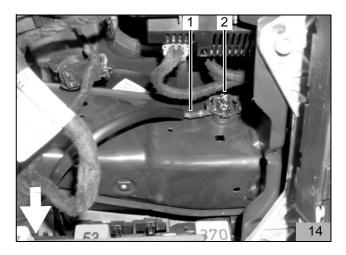
Lay the supplied positive distributor (15/1,2) to the standard positive post (15/3) using a 6 mm terminal lug as shown in the Figure 15 and to the central electrical system
