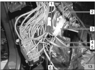
Connect the br cable (14/1; 13/2) 4.0 mm<sup>2</sup> to the standard earth point (14/2) using the supplied 6 mm terminal lug
